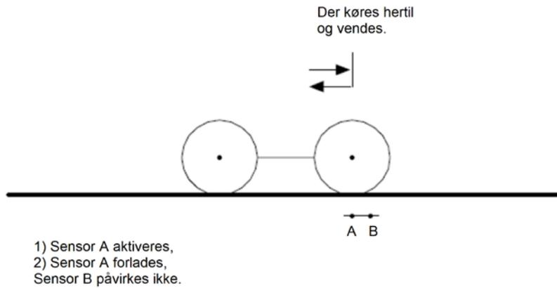
**Pendling på to sensorer**
